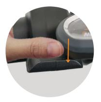
You can use the Easy-Start by pressing the trigger to start the motor without having to cycle. Once the bike is started, the motor will be activated by cycling and not by the trigger (in compliance with the current standard)
