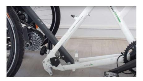
Put the bicycle frame on the hub between the frame plate and the washers. Tighten the two cap nuts with a 15 mm spanner or box wrench.
