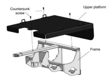
Unscrew the three dome head screws on the platform using a 4mm Allen key. Remove the upper platform from the frame to gain access to the hub. Store it in the box in the meantime. You will need it at the very end of the installation. Reposition the screws on the frame so that you do not lose them.
