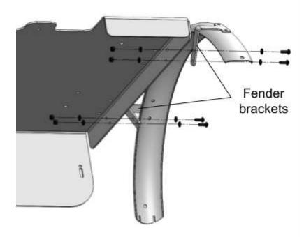
Step 2: Installing the platform on the B-Back
