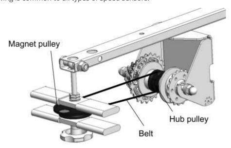
Insert the Adapt'Elec's components on the eyebolt: the spacer, then the magnet pulley on the spacer (with the magnet up), then the second M10 nut. Tighten this nut with the 17 mm Allen key.
