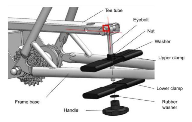
Once the correct height has been found, tighten the two nuts against each other using the two 17 mm spanners.
