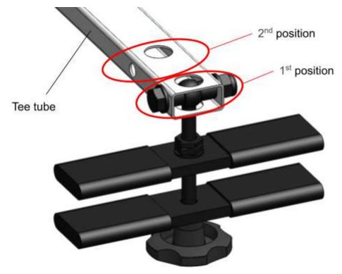
The B-Back was delivered to you with the clamp system in position 1. However, if something on your frame interferes with the positioning of the clamp system, you will need to move it to position 2. So, first you need to install the B-Back on the bike to test the clamp system.
