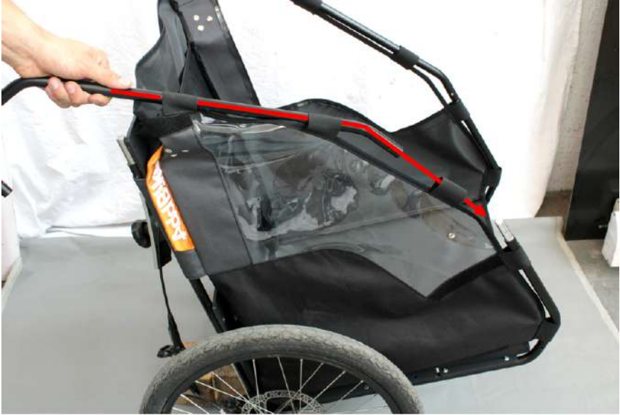
Illustration 9 - Inserting the upper tubes into the textile straps
