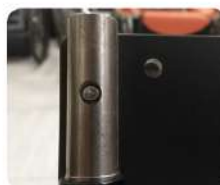
Figure 4 - Screws to be removed from the seat and backrest
