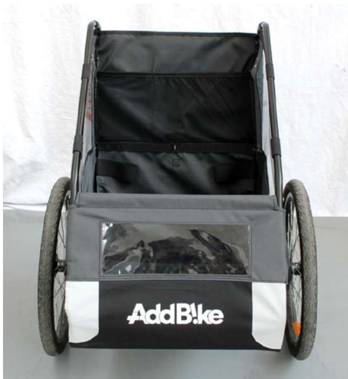
Illustration 17 – Assembly of the front textile on the module
