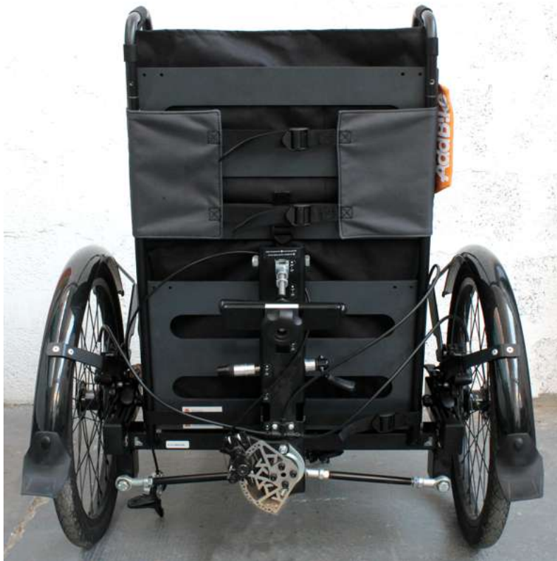
Illustration 14 - Tighten straps on the backrest of the AddBike+
