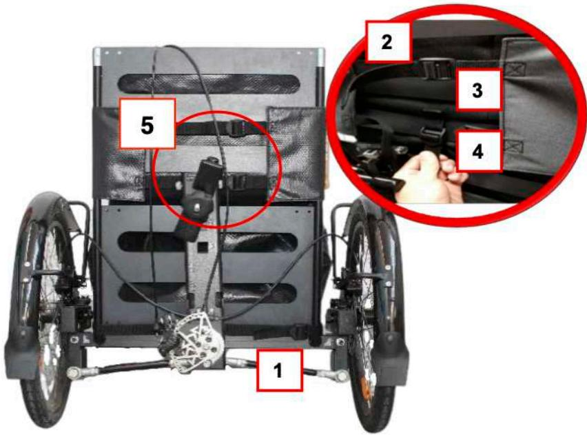
**EN** Tighten the fabric on both sides, centering the fabric on the backrest as much as possible.
