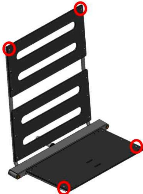
EN Install the compact slat with 4 screws BHC M5x20 at the bottom of the two tubes (as shown on the right).
