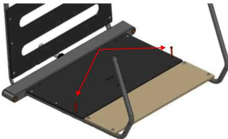
EN Insert the assembly just built into the seat by fastening the 2 previously removed screws
