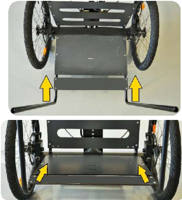
Illustration 5 - Insertion of front tubes into the seat
