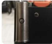
Illustration 4 - Screws to be removed from the seat and backrest
