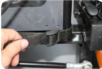
Illustration 8 - Tightening of the lower strap of the textile
