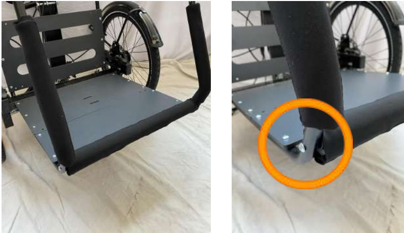
Illustration 8 - Installation of the Crossbar
