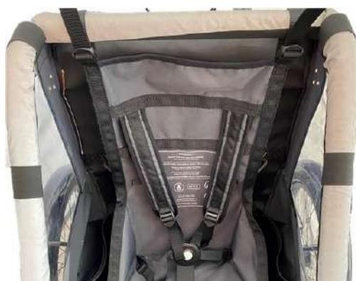
**EN** To secure the front textile insert the straps of the hammock on each side. Proceed by positioning and screwing in the transverse bar as shown in the bottom image. The two screws required are BHC M5x30.
