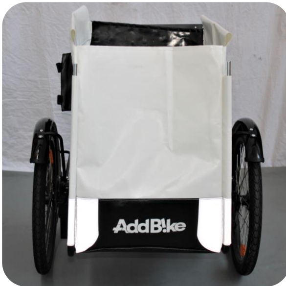
Figure 7 - Insertion du textile
