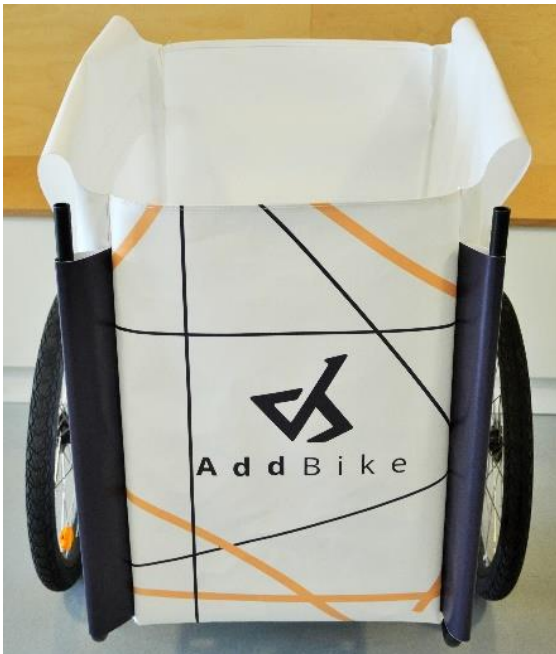
Figure 7 - Insertion du textile
